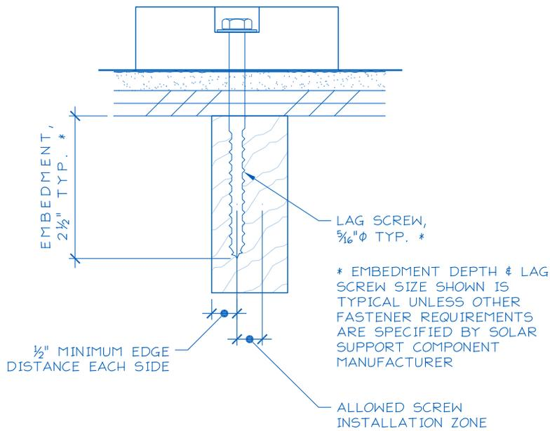
**Figure 3. Typical Anchor with Lag Screw Attachment.**
