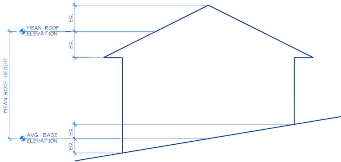
**Figure 5. Definition of Mean Roof Height.**
